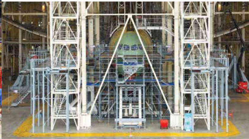
Toulouse: scaffolding for Airbus A350-900 resistance tests.
